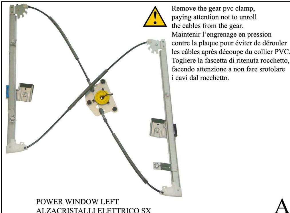
Remove the gear pvc clamp,
